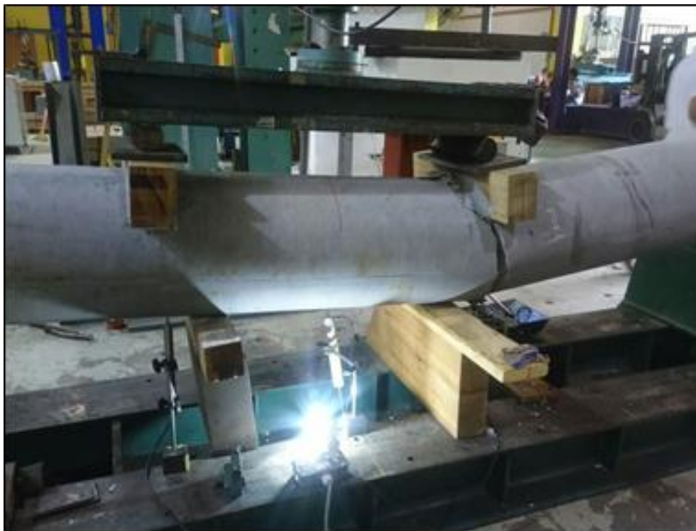
Figure 5(b) Failure Test Mod under Bending Test for SC400 Ø (pile body)
